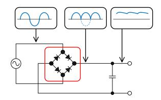
Figure 2-3. Full-wave Rectifier Circuit
