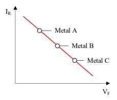
Figure 3-9. Characteristics Depending on the Metals
