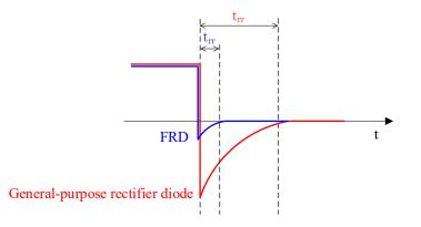
Figure 3-1. Comparison of Reverse Recovery Time, t<sub>rr</sub>
