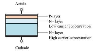
Figure 2-5. PN Junction (P-layer / N-layer)
