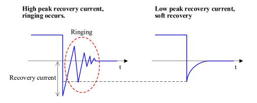
Figure 3-3. FRD Reverse Recovery Time, t<sub>rr</sub>
