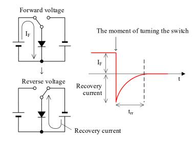
Figure 2-9. Reverse Recovery Time, t<sub>rr</sub>
