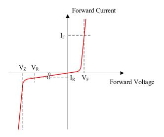
Figure 2-8. Static Chracteristics of Diodes
