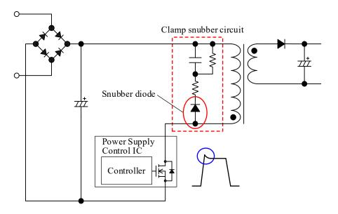
Figure 3-4. Clamp Snubber Circuit
