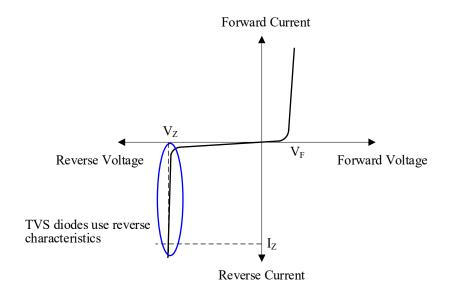
Figure 3-6. Diode Static Characteristics
