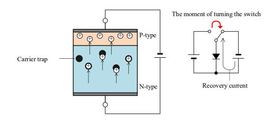
Figure 3-2. Carrier Trap
