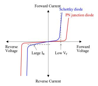
Figure 3-7. Static Characteristics Comparison
