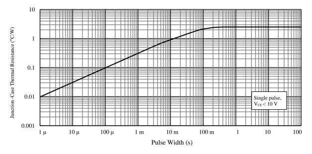
Figure 19. Typical Transient Thermal Resistance Characteristics
