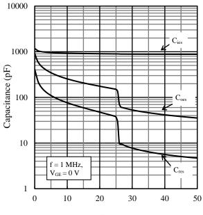
Collector–Emitter Voltage,  $V_{CE}(V)$
