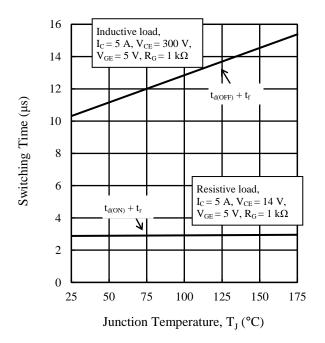
Figure 18. Typical Characteristics: Switching Time vs. T<sub>J</sub>
