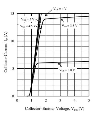
Figure 7. Typical Characteristics:  $I_C$  vs.  $V_{CE}$   $(T_J=-40\ ^\circ C)$
