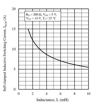
Figure 15. Typical Characteristics: I<sub>SCIS</sub> vs. L
