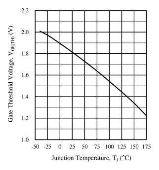
Figure 13. Typical Characteristics:  $V_{GE(TH)}$  vs.  $T_J$ ( $V_{CE} = 10$  V,  $I_C = 1$  mA)
