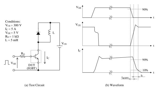
Figure 3. Switching Time Test in Inductive Load
