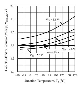
Figure 12. Typical Characteristics:  $V_{CE(SAT)}$  vs.  $T_{\rm J}$   $(I_C$  = 10 A)
