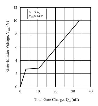
Figure 17. Typical Characteristics: V<sub>GE</sub> vs. Q<sub>G</sub>
