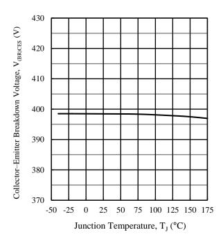
Figure 14. Typical Characteristics:  $V_{(BR)CES}$  vs.  $T_J$ ( $V_{GE} = 0$  V,  $I_C = 2$  mA)
