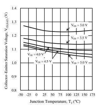
Figure 11. Typical Characteristics:  $V_{CE(SAT)}$  vs.  $T_{J}$   $(I_{C}=5\ A)$
