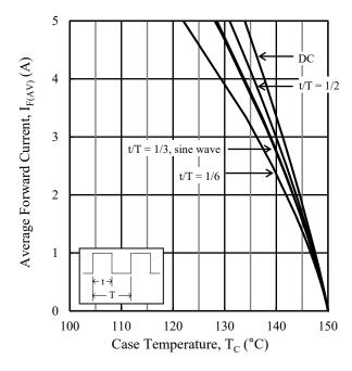
Figure 1.  $I_{F(AV)}$  vs.  $T_C$  ( $T_J = 150$  °C,  $V_R = 0$  V)
