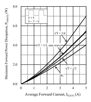
Figure 3.  $P_{F(MAX)}$  vs.  $I_{F(AV)}$  ( $T_J = 150$  °C)
