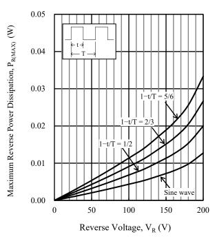
Figure 4.  $P_{R(MAX)}$  vs.  $V_R$  ( $T_J = 150$  °C)
