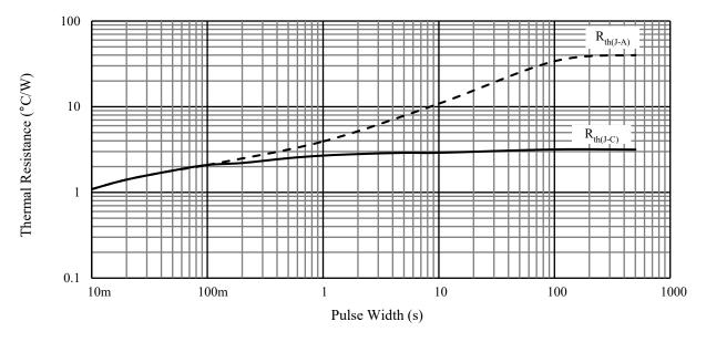
Figure 7. Typical Transient Thermal Resistance Characteristics
