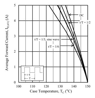
Figure 2.  $I_{F(AV)}$  vs.  $T_C$  ( $T_J = 150 \, ^{\circ}\text{C}$ ,  $V_R = 200 \, \text{V}$ )
