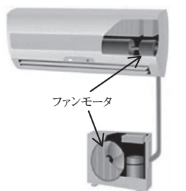
(a) ルームエアコン内観図 Inner view of room air conditioner
