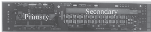
Fig. 14. A total of 36 super-junction FETs are mounted on the back of Fig. 20 to suppress the positive temperature coefficient.
