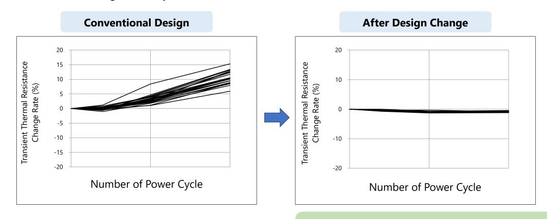
High reliability against thermal stress is maintained in flow mounting (MSL1) as well!
